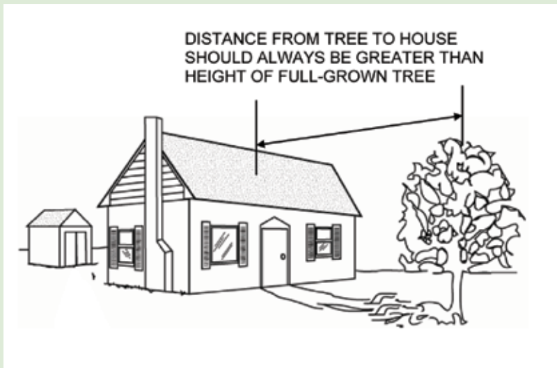
Figure 4-45. FEMA recommends that the distance between a tree and your house should always be greater than the height of the full-grown tree. This is to prevent trees from falling on the roof. 32
